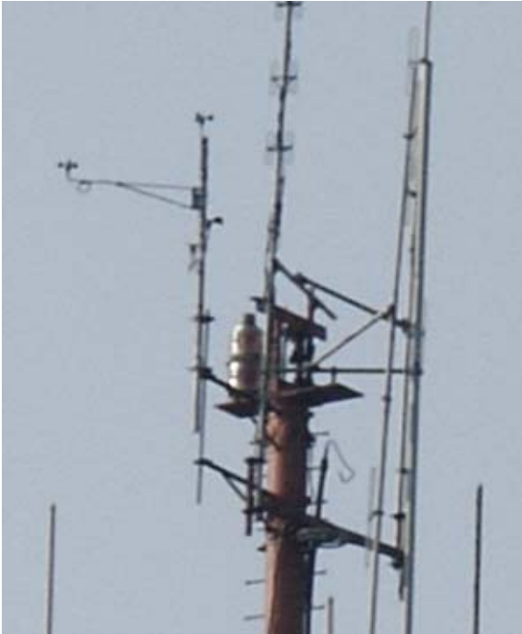
Figure 2 - Instrumentation at top of Yankee Network Tower – note the anemometers on the left (horizontal boom and at the top of the left-hand vertical tube).
