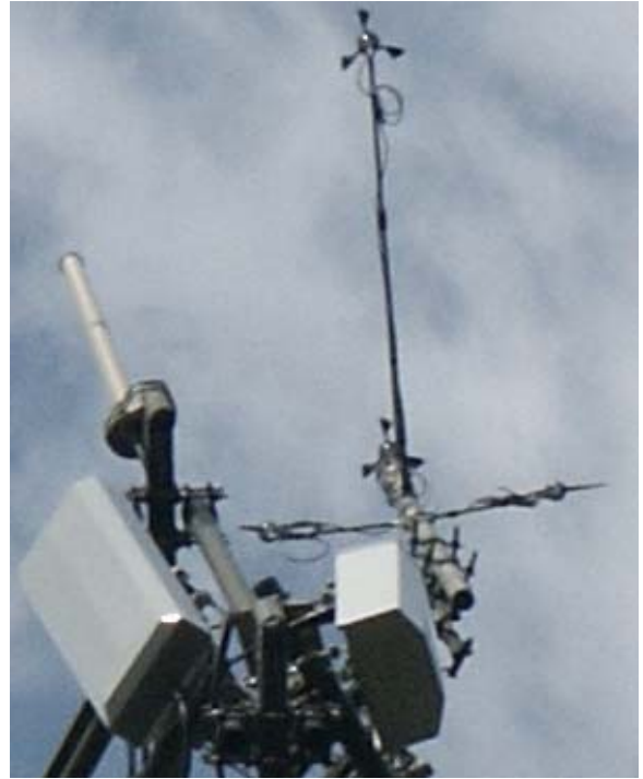
Figure 3 – Bottom view of sensor array, anemometer is at photo top and wind vanes are mounted on the shorter side booms.
