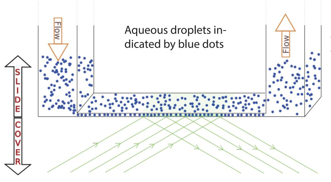
Designed to be used in through objective total internal reflection fluorescence microscopy for reduced background and ease of use.
