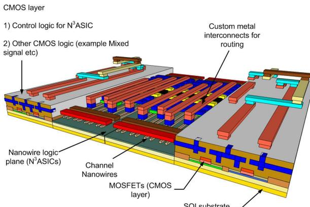
Figure 2 A Nano-CMOS 3-D integrated fabric
