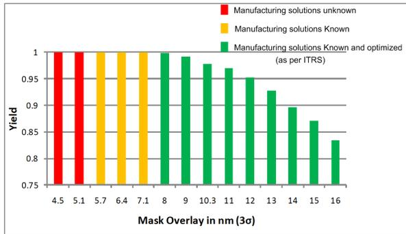
Figure 7 Yield vs. Overlay for 3D integrated fabric
