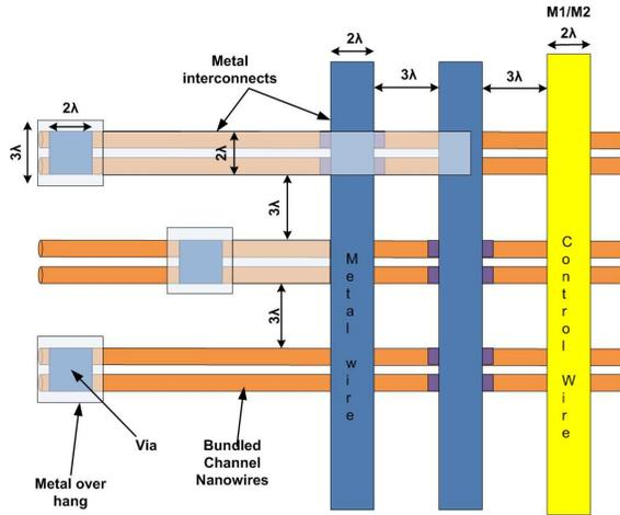
Figure 1 NW design rules for 3-D integration
