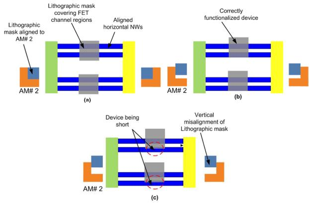
Figure 6 Mask registration during functionalization step
