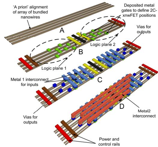
Figure 3 A simplified manufacturing sequence
