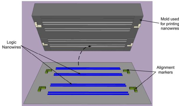
Figure 4 Nanowires and the alignment markers in the same mold for NIL technique
