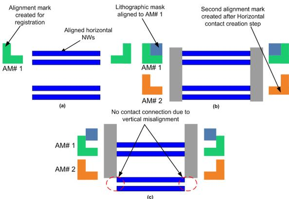
Figure 5 Mask registration during contact creation step
