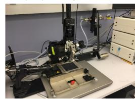
Placement accuracy 5  $\mu$ m Components from 0.125 mm x 0.125 mm to 100 mm x 100 mm Working area up to 450 mm x 234 mm Supports wafer/substrate sizes up to 200 mm
