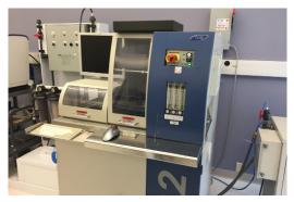
Work piece size: up to 200mm x 200mm Indexing: resolution/accuracy is 0.2 µm/1.5 µm Cut Depth: resolution/accuracy is 0.2 µm/2.0 µm
