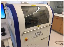
Diameter of UV laser beam 20µm Resolution of scanfield 2µm Repeatability +/- 2µm Surface structures down to 75µm Max material size 9" x 12" x 0.27"
