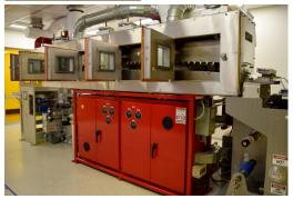
The Frontier coater is a versatile tool enabling solution-based coatings over a range of viscosity and thicknesses for the development of advanced coatings.
