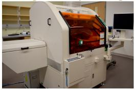
The web-based pick and place/die attach tool provides users with an advanced capability to develop methods for flexible-hybrid electronic circuit integration and system prototyping.
