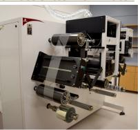
This custom built atmospheric slitter/laminator tool enables final sizing, slitting and lamination steps to be completed for prototyping and test.
