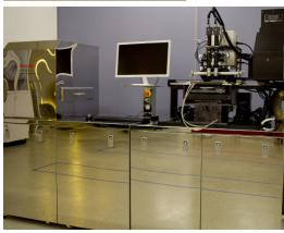
The Nanonex Nanoimprint Lithography tool provides state-of-the-art capability for patterning, alignment, and direct printing of multiple materials for printed electronics.
