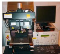
A UV mask aligner and exposure system with split screen stereo camera alignment system capable of both front and back side alignment of from 2" to 6" diameter substrates.
