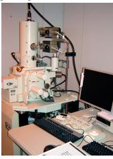
The Electron Beam Lithography system is based on a JEOL JSM-7001F Thermal Field Emission SEM equipped with a Nabity Nanometer Pattern Generation System which supports e-beam lithography and an image database.
