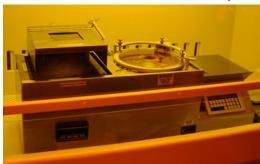
The Brewer Science CEE 100CB Spin Coater and Hot Plate is capable of storing up to 10 spin regimes which may include spin speed ramp rate, stepped spin speeds, and a nitrogen float or vacuum hot plate contact mode for photoresist curing. Chucks for substrates from 1" to 6" diameter are available.
