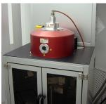
gen, methane, sulphur hexafluoride, trifluoromethane, oxygen, argon, and nitrogen. The STS Vision 310 Plasma Enhanced Chemical Vapor Deposition system is equipped with a patented frequency generator that allows for the deposition of low stress films. It is
