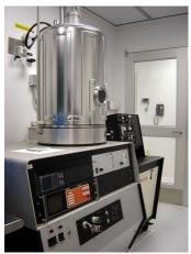
The CHA SE-600 electron beam evaporator with a 4 pocket hearth has been retrofitted with a cryopump to decrease the pumping cycle time. More than twenty different metals can be evaporated including gold, platinum, palladium, silver, copper, aluminum, nickel, and titanium.
