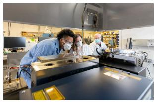
State of the art MALDI-TOF instrument for high sensitivity measurement of limited sample quantity (routinely low fmol amounts). 2 kHz laser repetition rate enables rapid data acquisition at high resolution and mass accuracy. Laser technology enables focus to 10  $\mu m$  for high resolution spatial imaging applications.
