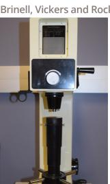
The Brinell, Vickers and Rockwell Hardness Testing Unit (EBVR) consists of a hardness testing machine that determines the three main types of hardness (Brinell, Vickers and Rockwell).
