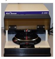
The Alpha D-500 stylus profiler allows high resolution characterization of 2D surfaces. The measurements can be used to ascertain step height, roughness, bow, and shape of a piece, as well as measurement of stress. The device also allows high resolution visualization of surface features. Such measures are used in a variety of fields, including materials research and medical devices.
