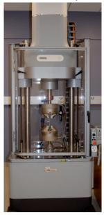
The ElectroPuls 10000 can test material properties under large linear and torsion loads and at high strain. Using the system a material or device's material and fatigue responses can be tested to determine its performance and validate its manufacturing process.
