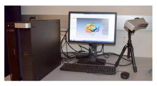
The Capture 3D scanner allows rapid characterization of the surface geometry and shape of an object. The scanner allows rapid creation of a digital model of a physical object. Industrial uses include fields as varied as quality control, orthotics, and prosthetics. Though not as accurate as a coordinate measuring machine, the 3D scanner requires no physical contact.
