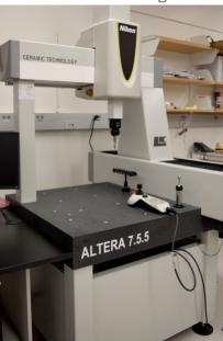
The Nikon Altera 7.5.5 allows high precision characterization of device geometry in critical to function locations. Using a 5-axis measuring system and a number of probe options, the system measures with volumetric accuracy on the order of 1.8 microns, allowing a designer to confirm part dimensions to tight tolerances.
