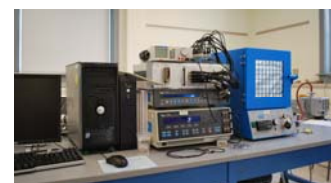
Photovoltaic cell fabrication and analysis unit and the impedance spectroscopy unit for proton conductivity measurement, part of the UMass Amherst "Charge Transport Laboratory."
