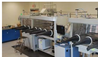
Photovoltaic cell fabrication and analysis unit and the impedance spectroscopy unit for proton conductivity measurement, part of the UMass Amherst "Charge Transport Laboratory."
