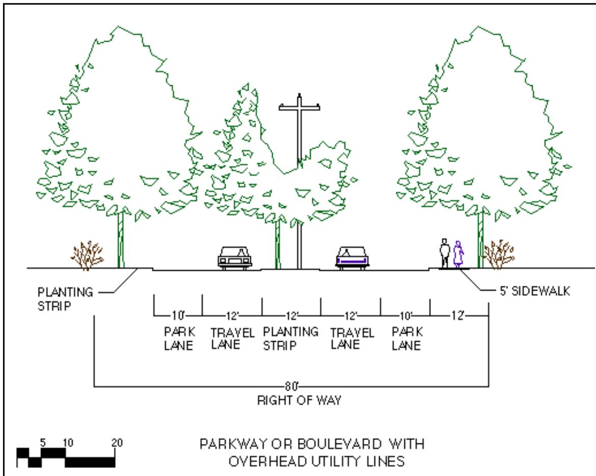
FIGURE 85 - Cross section of a boulevard street with overhead utility lines along center planting strip.
