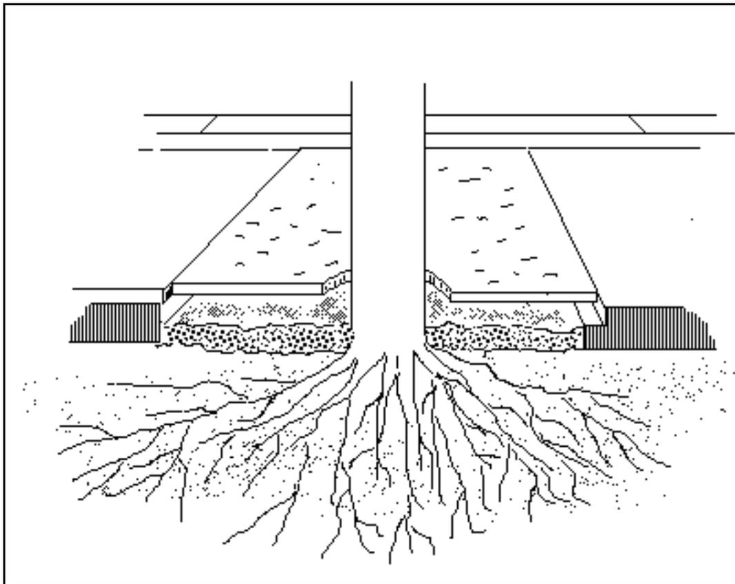
FIGURE 90 - Planting well with cover allowing for deeper rooting.
