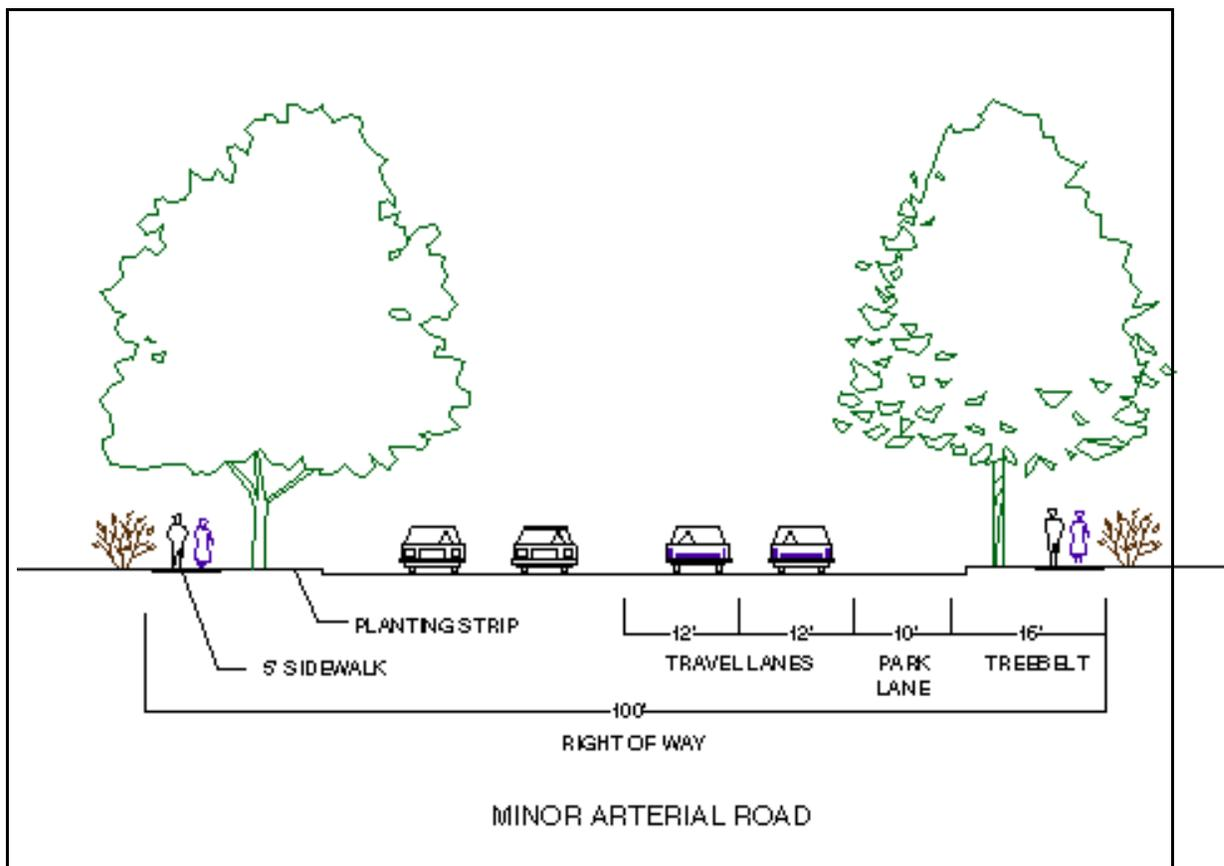
FIGURE 36 - Cross section of a minor arterial road .
