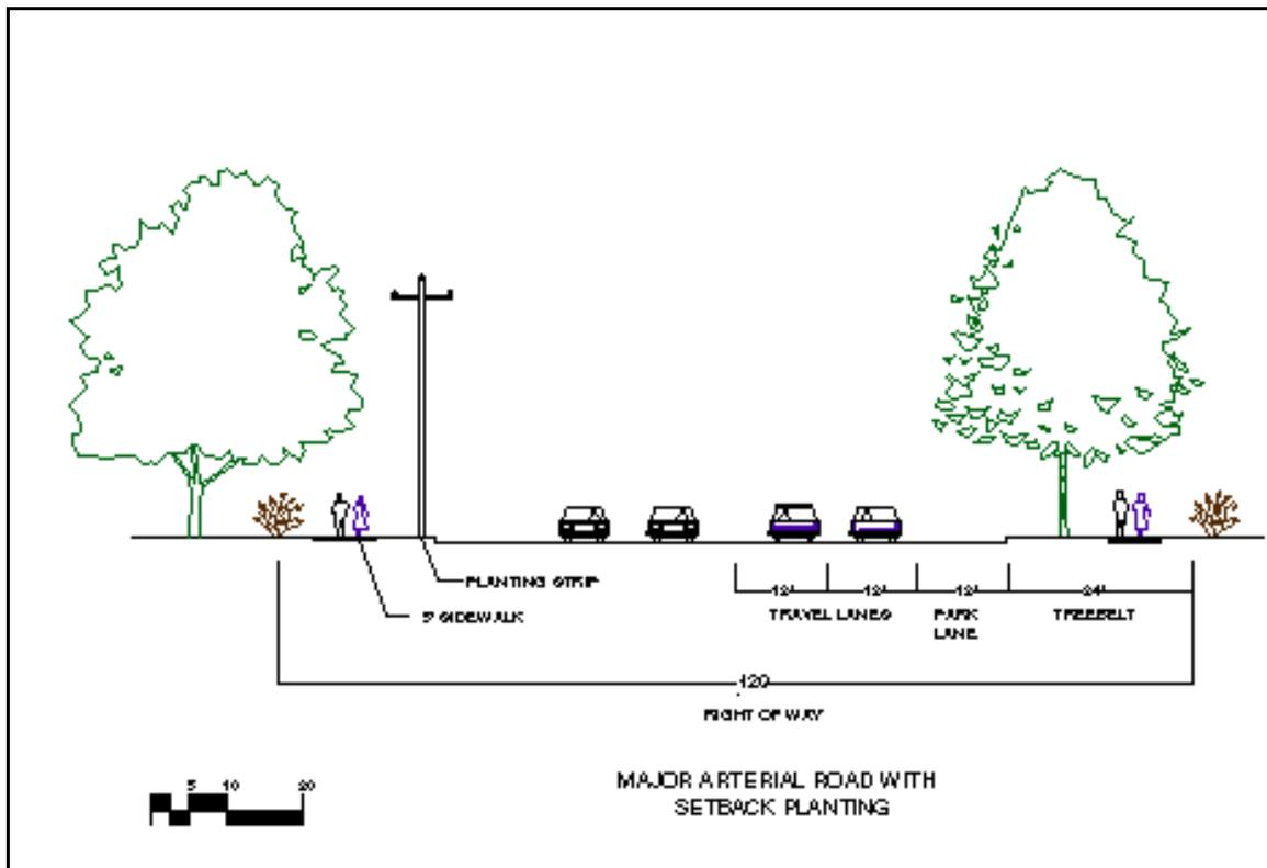
FIGURE 63 - Cross section of a major arterial road with setback planting.
