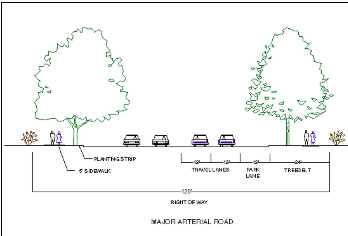
FIGURE 34 - Cross section of a major arterial road.
