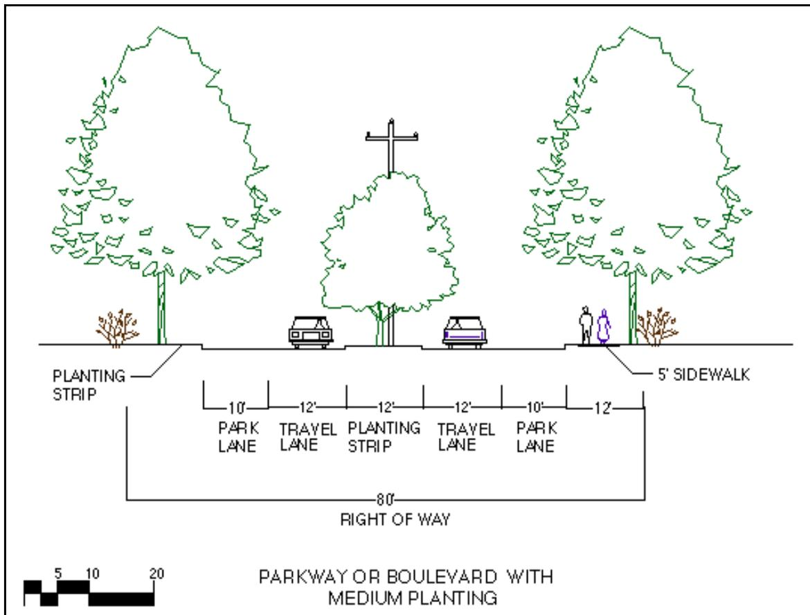
FIGURE 88 - Cross section of a boulevard street using smaller tree species along center planting strip.
