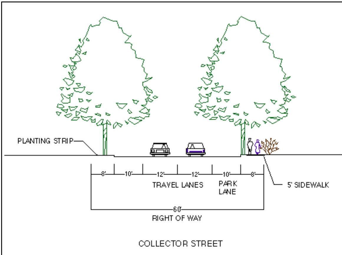
FIGURE 37 - Cross section of a collector street .
