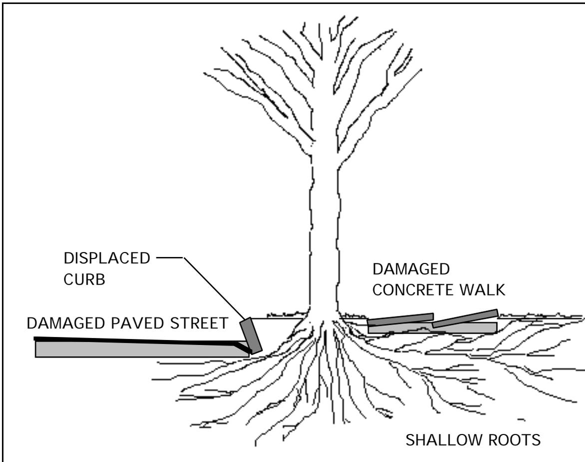
FIGURE 60 - Tree roots and damage to surface infrastructure.
