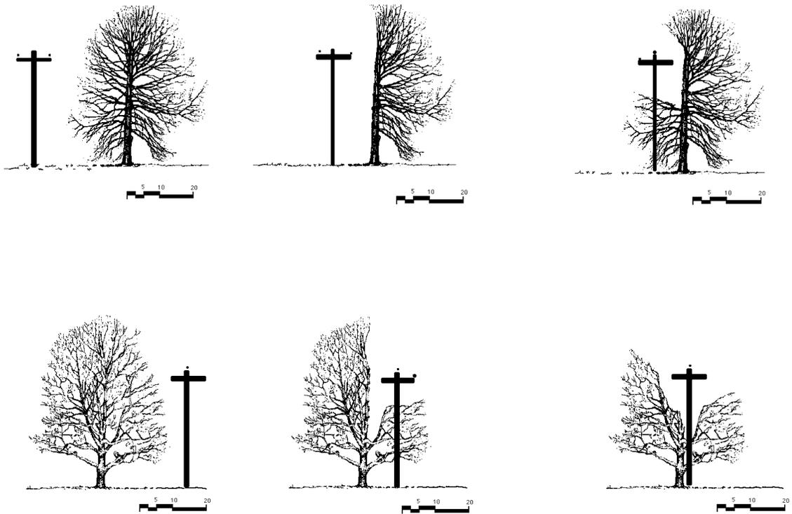
FIGURE 24 - Trees trimmed for clearance from utility lines.
