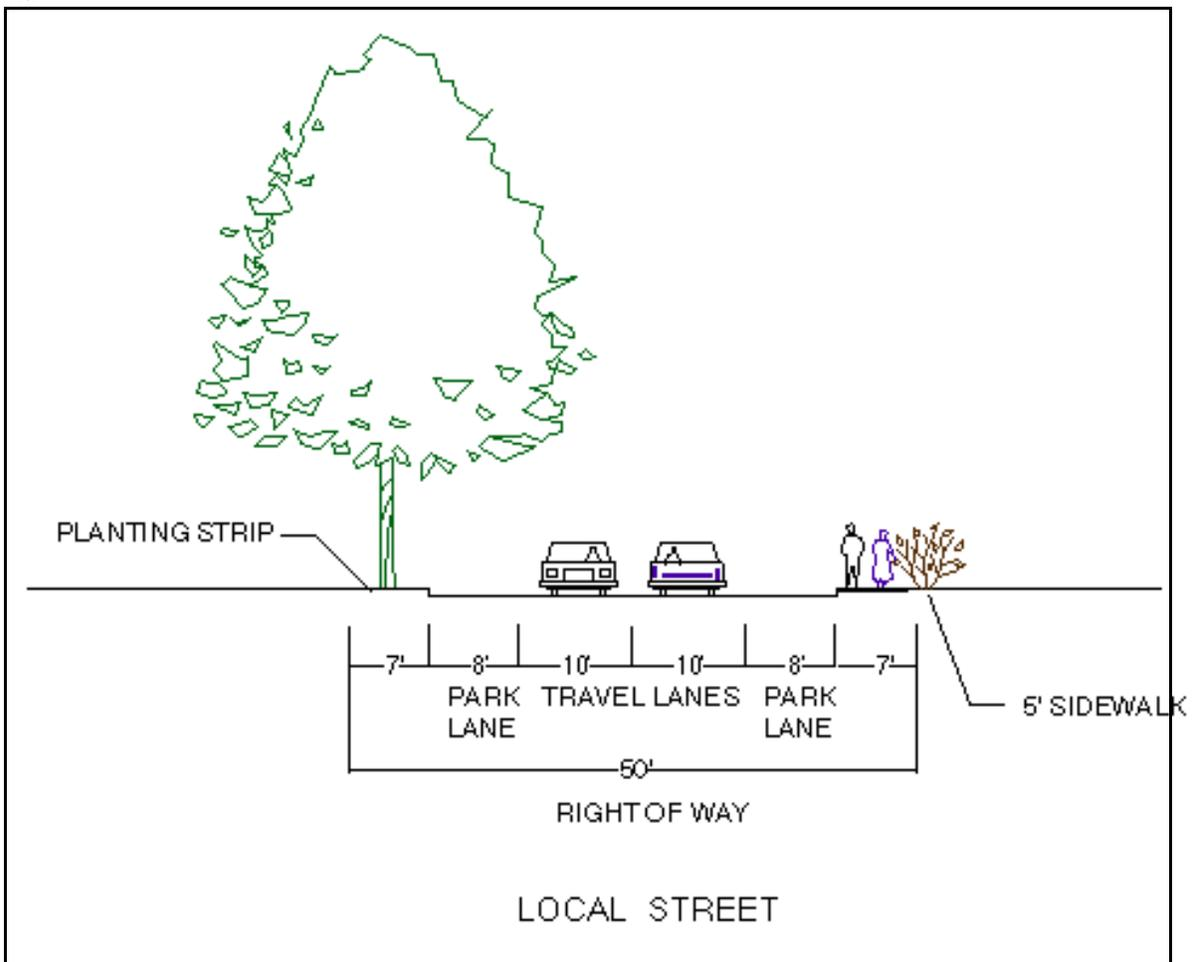
FIGURE 38 - Cross section of a local street .
