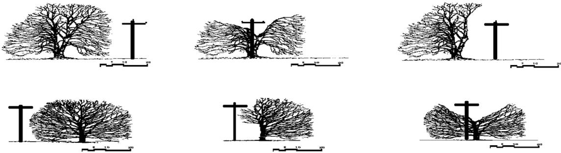
FIGURE 25 - Trees trimmed for clearance from utility lines.
