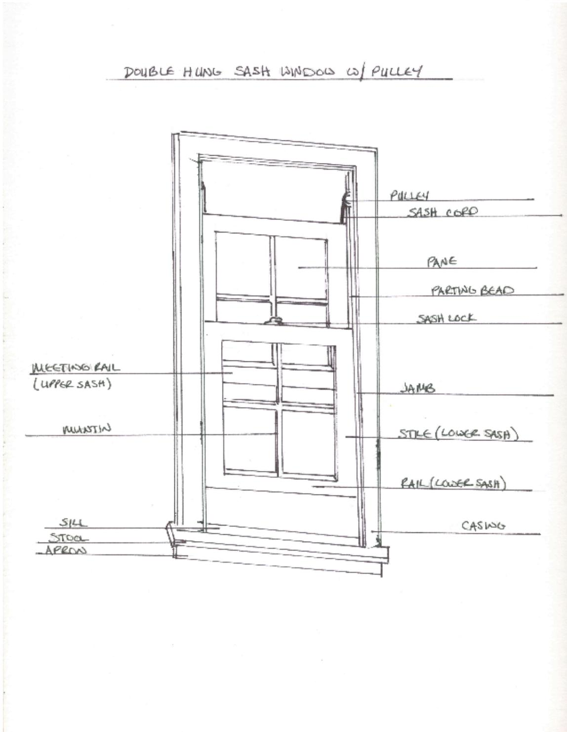
Figure 1 Typical Double-Hung Window
