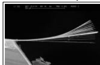
Figure 3: Scanning electron micrograph of an array of thermally-actuated probes.
