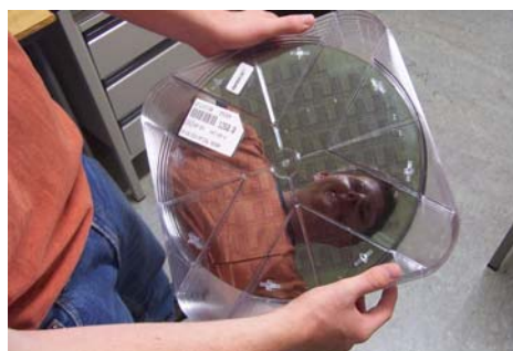
Fig. 2. Photograph of nanocrystal memory devices fabricated in collaboration with Intel Corporation on 300 mm substrates in a conventional silicon ultralarge scale integrated (ULSI) process.
