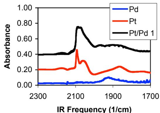
Figure 1. IR spectra of CO adsorbed on dendrimer-templated catalysts.
