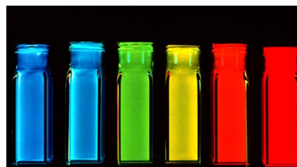
Fig. 2. CdSe quantum dots luminescing from blue to red as a function of increasing dot size (1.5- 8nm). (Photograph by Felice Frankel)
