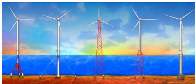
Figure 10: Example support structure options for offshore wind turbines.
