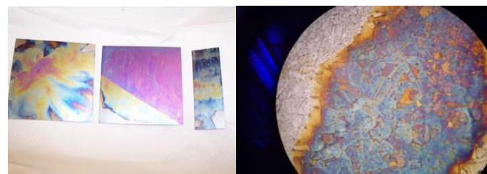
Figure 2. Anodized titanium pieces (left) and metal surfaces (right, Ni shown) prepared for an outreach module. The image on the right is shown as observed under the optical microscope at a magnification=200x.
